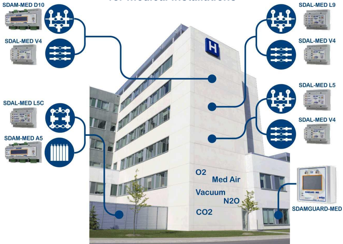
***Medical gases pipeline system with 2nd stage pressure regulators on each floor***
